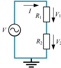
$$I = \frac{V}{R_1 + R_2} \quad V_1 = I \cdot R_1; \quad V_2 = I \cdot R_2$$
