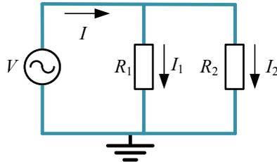
$$I_1 \cdot R_1 = I_2 \cdot R_2; \quad I = I_1 + I_2$$
